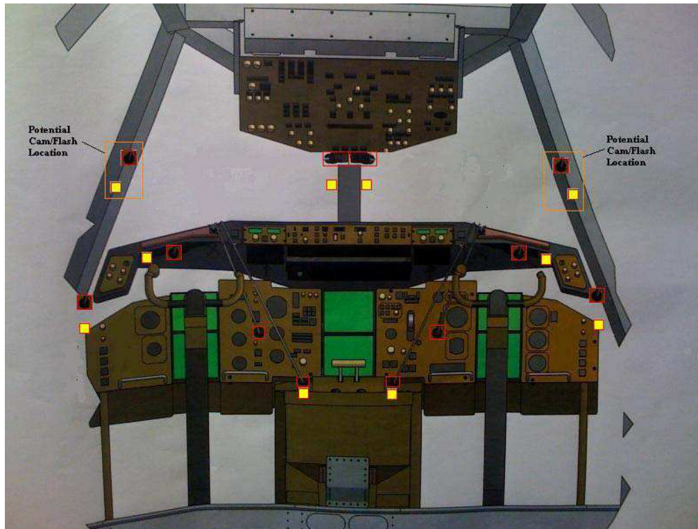
Figure 20. IFD SE Camera and Illuminator Locations
